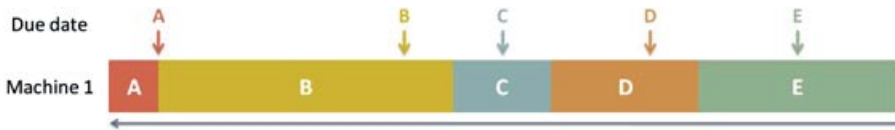
Figure 3 The earliest due date (EDD) algorithm: from the earliest to the latest due date.
