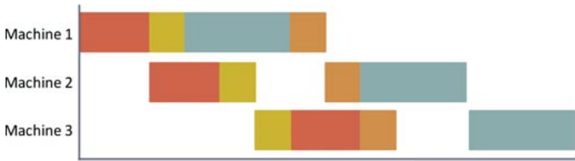
Figure 1 The machine planning board. Bars of a length proportional to the required processing time represent job operations. Different colors indicate different jobs.
