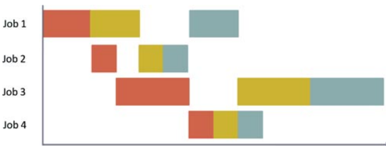
Figure 2 The modified machine planning board. Bars of a length proportional to the required processing time represent job operations. Different colors indicate different machines.
