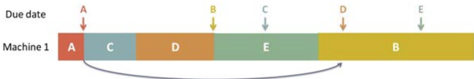
Figure 4 The Moore–Hodgson (MH) algorithm. The first step is the EDD algorithm. The second step consists of reporting the longest jobs at the end.
